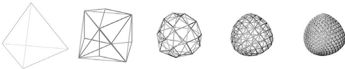
Figure 2 Tetrahedral control mesh (left), converging on its limit surface (right), after subsequent subdivision operations.
