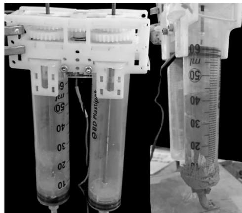
**Figure 1.** The autonomous syringe deposition device, suitable for carriage by an aerial robot.
