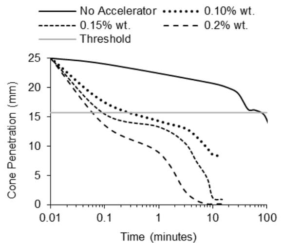
**Figure 2.** Cone penetration of the 0.33 w/c ratio, 1.5% wt. of cement superplasticiser mix with added 1:1 aluminium lactate and diethanolamine accelerator by 0.10, 0.15 and 0.20 % wt. of cement. The x-axis has a logarithmic scale.
