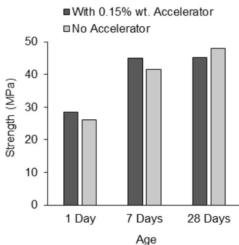
**Figure 3.** Compressive strength of the chosen cement mix.
