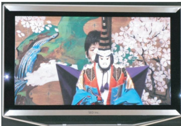
**Figure 13** A prototype 55-in. SED manufactured consisting of (H)1920  $\times$  3  $\times$  (V)1080 pixels. The display showed high brightness ( $450\ \text{cd}/\text{m}^2$ ) with high luminous efficacies of 5–7 lm/W and rapid response times of  $<1\ \text{ms}$  (Courtesy of M. Nakamoto, CEATEC-Japan, 2006 with kind permission of SED Corp.)
