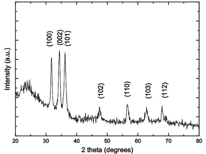
Fig. 3. XRD spectrum of the intercalated ZnO thin film.
