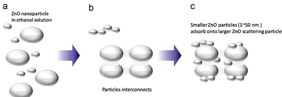
Fig. 2. Proposed growth mechanism of the intercalated ZnO thin films. (a) Initial formation of the ZnO particles, (b) larger ZnO particles bind from the seed layer growing ZnO and (c) smaller ZnO nanoparticles adsorb onto the larger ZnO particles, increasing film connectivity.
