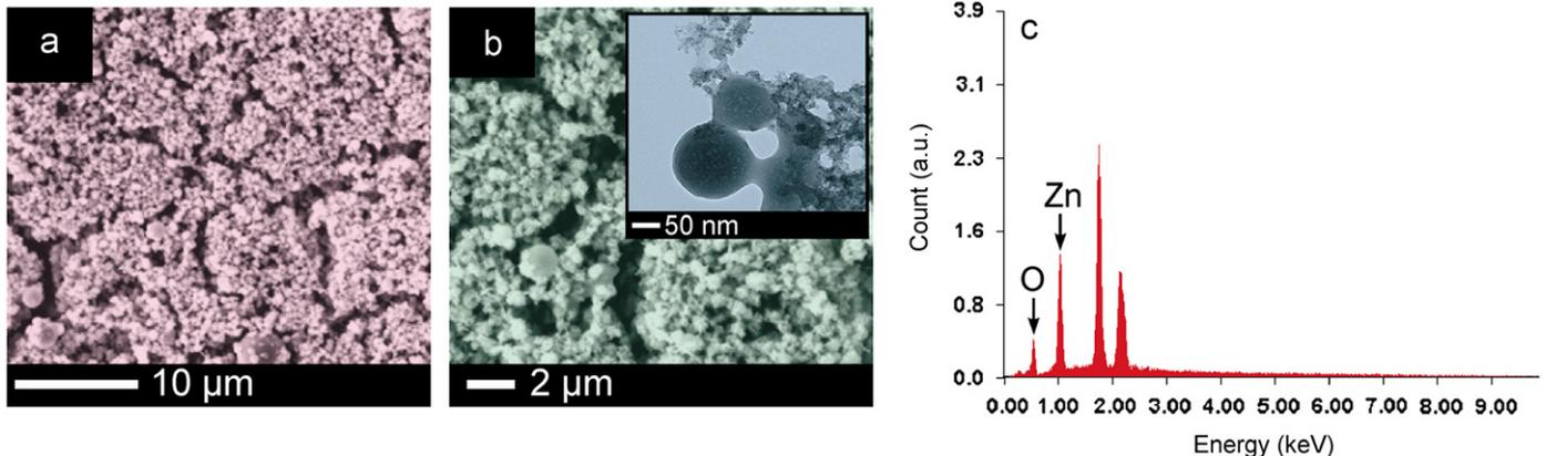
Fig. 1. Morphology of the intercalated ZnO thin films. (a) A scanning electron micrograph of an intercalated ZnO thin film at low magnification (scale bar: 10  $\mu$ m). (b) An SEM micrograph at higher magnification highlighting the variation in nanoparticle size within the film (scale bar: 2  $\mu$ m). The inset shows the corresponding TEM image (scale bar: 50 nm). (c) EDS compositional analysis of the film.
