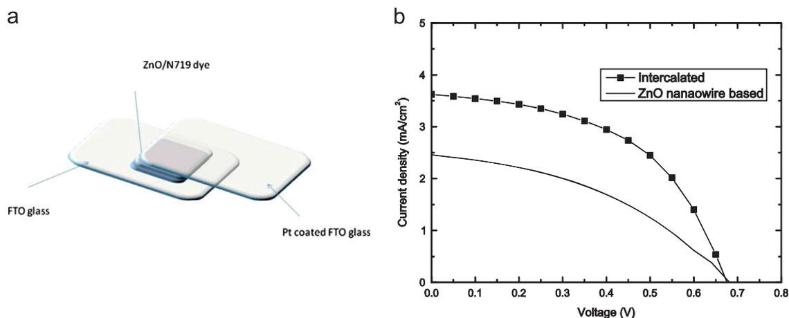
**Fig. 4.** Intercalated ZnO integration in DSSCs. (a) Illustration of the DSSC construction and (b)  $J$ - $V$  of an intercalated ZnO photoanode DSSC (■) compared to a ZnO nanowire cell of nominally equivalent construction.
