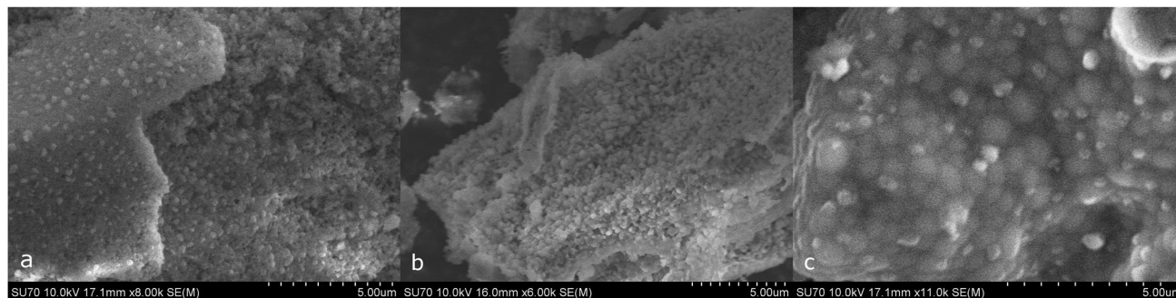
Fig. 7 SEM images of \text{Na}_2\text{CoSiO}_4 with NaCl removed before annealing at (a) 500, (b) 700 and (c) 900 °C under flowing \text{N}_2 .
