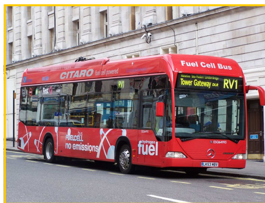
Figure 2: A fuel cell bus powered by hydrogen being trialled in London.
