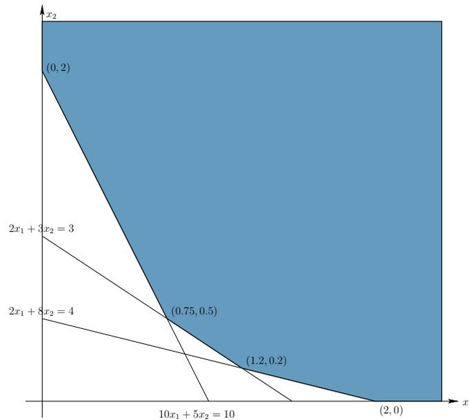
Figure 1: The region, shaded, for which all the feasible solutions to Example 1 must lie. The region has four extreme points:  $(0, 2)$ ,  $(0.75, 0.5)$ ,  $(1.2, 0.2)$  and  $(2, 0)$ . The lines  $x_1 = 0$  (for  $x_2 \geq 2$ ) and  $x_2 = 0$  (for  $x_1 \geq 2$ ) are **extreme rays**. This feasible set is unbounded.
