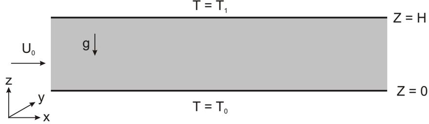
Figure 6.1: Fully Saturated Porous Layer with Throughflow.
