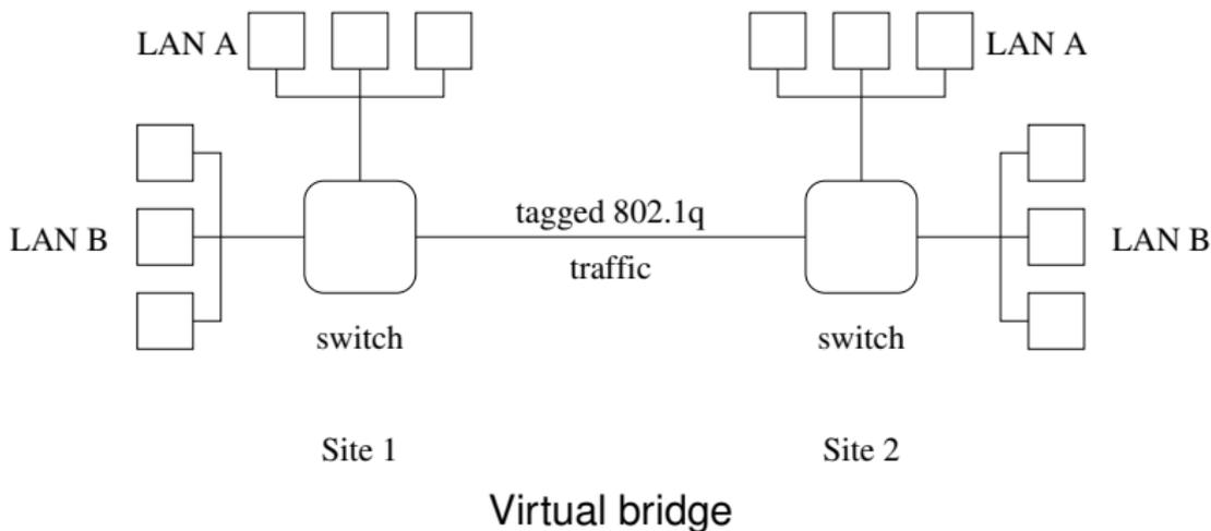
A tag is an extra four byte header containing a *Virtual LAN Identifier* (VID), a 12 bit integer;
