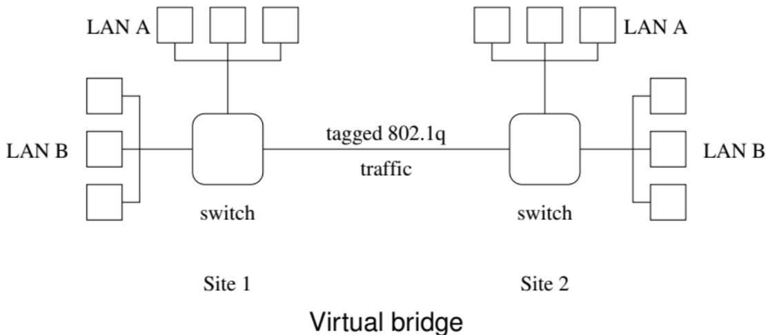
The frame type in the physical layer (typically Ethernet) is changed from 0800 to 8100 to indicate a tagged packet;
