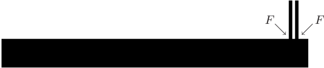
Fig. 10 Design for the S-history single-run-global minimum of S(\mathbf{x}) ( e ) by ESO on a refined initial design domain having V(\mathbf{x}) = 99 , C(\mathbf{x}) = 392 , S(\mathbf{x}) = 38671
