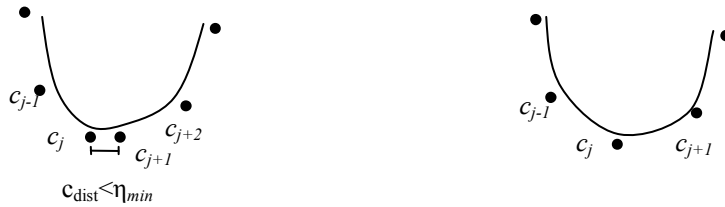
(a) Before two control points to be merged, c_j and c_{j+1} (b) New merged control point c_j
