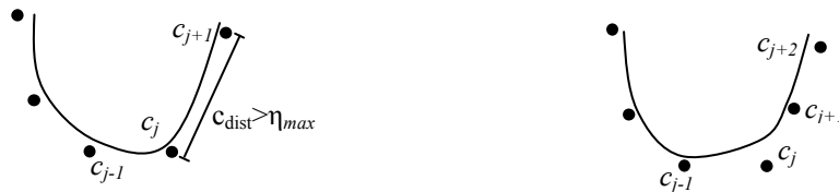
(a) Before a control point has been inserted (b) After a control point has been inserted
