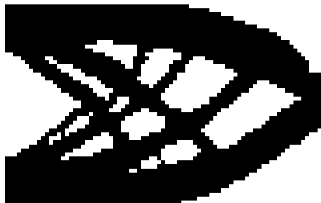
Figure 3. Solution found on mesh of 80 \times 50 elements. The buckling constraint is set to c_s = 0.9 and the compliance constraint c_{\max} = 35 . A volume of 0.6255 is attained. Similarly to Figure 4 the buckling constraint c_2 is active and the compliance constraint c_1 is not.
