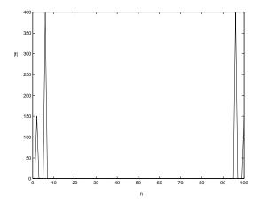
The vector  $|f_j|$  has four peaks at j = 2, 6, 96, 100 with corresponding amplitudes of 150, 400, 400 and 150.
