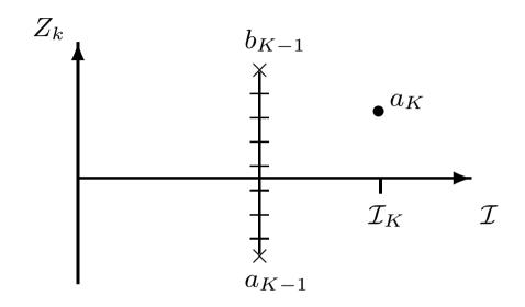
Before leaving analysis K-1, we set up a grid of points for use in numerical integration over the range  $a_{K-1}$  to  $b_{K-1}$ .
