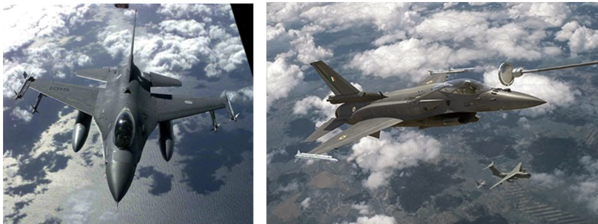
(a) An F-16A from the Portuguese Air Force prepares to refuel from a KC-10 via a flying boom. (b) A conformal air refuelling tanker/system (CARTS) was developed to enable probe-drogue refuelling.
