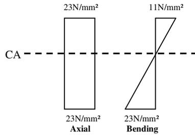
**Figure 13:** Axial and Bending moments generated in deck due to temperature change
