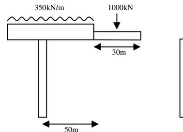
**Figure 11:** Maximum hogging experienced in deck during launching
