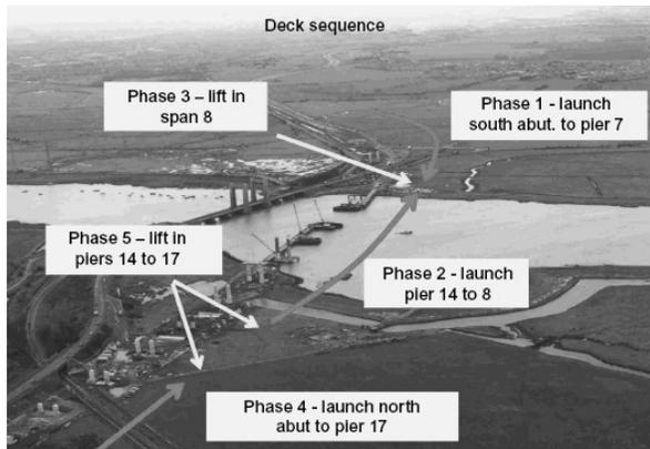
**Figure 9:** Steelwork erection phases - Ref. [3]
