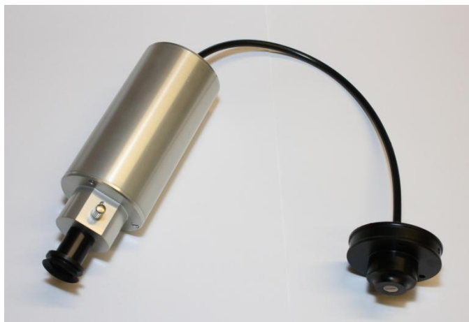
Figure 2.5: light guide and housing
