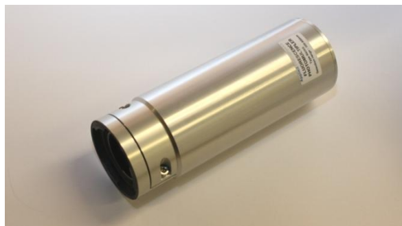
Figure 2.7: breech lock fitting mounted on the fluorescence detector
