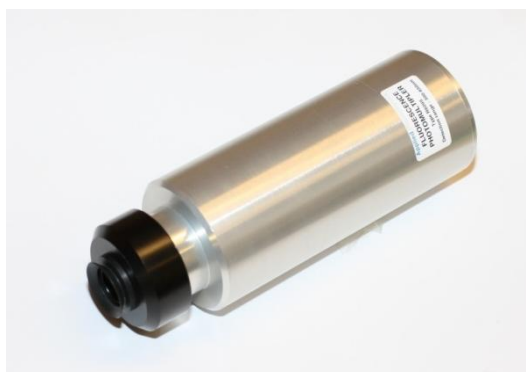
Figure 2.2: filter holder mounted on the detector
