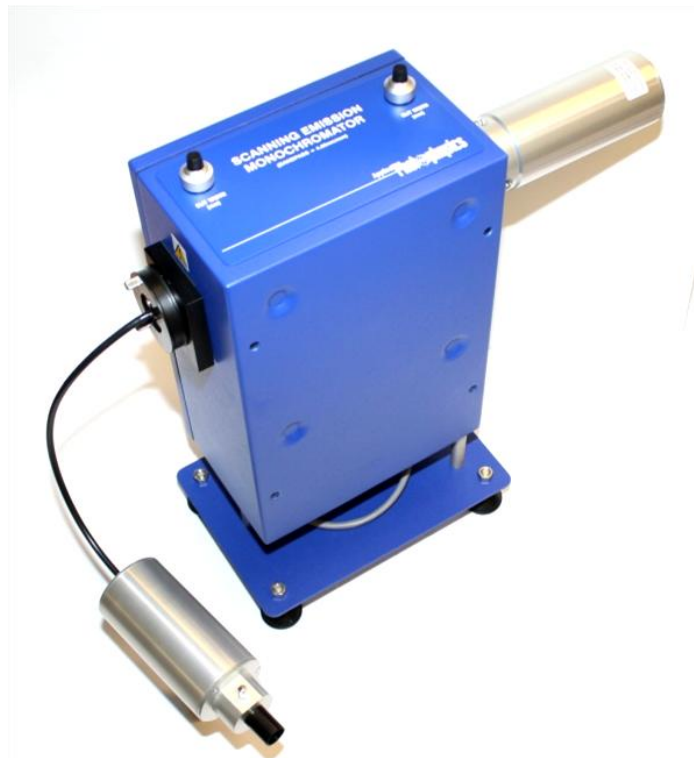
Figure 1.1: fluorescence detector and light guide mounted on the emission monochromator
