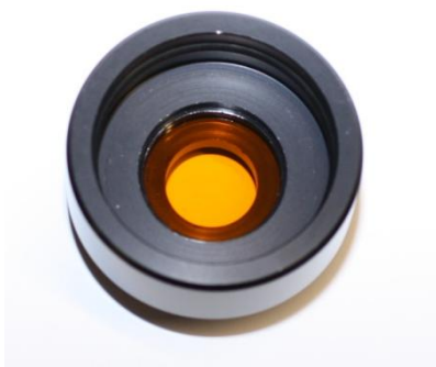
Figure 2.1: filter mounted within the filter holder
