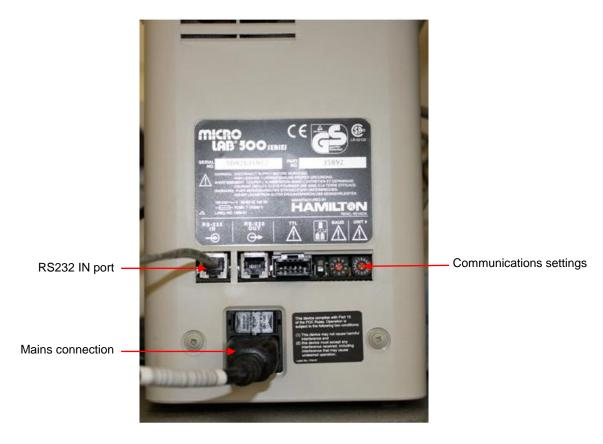
Figure 3.1: electrical connections to the CS/TT
