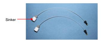
Figure 3.7: tubing between the titrator and reservoir or waste
