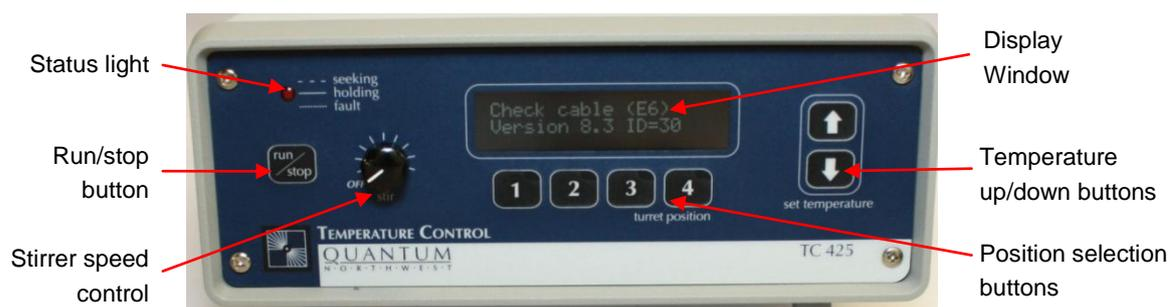
Figure 3.1: the CS/PCM electronics unit front panel
