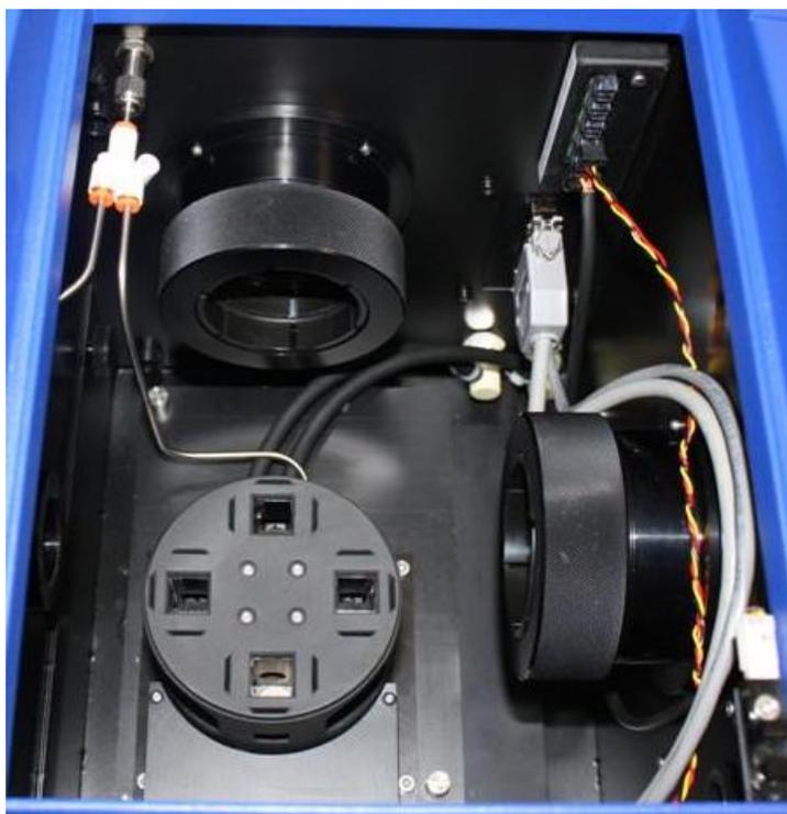
Figure 2.3: interior of the SHU with the turret in place
