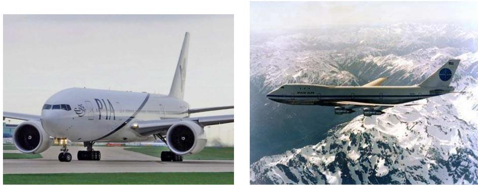
Figure 8.5: Trends in aircraft design: the Boeing 777 has two engines providing almost as much thrust as the four engines of the Boeing 747, a quieter, more fuel-efficient solution.
