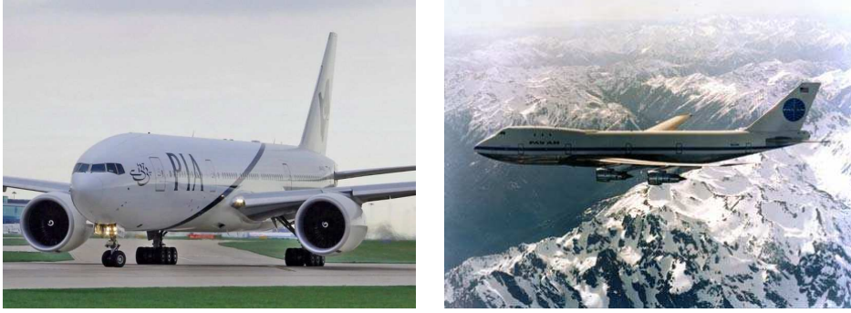
Figure 7.2: Trends in aircraft design: the Boeing 777 has two engines providing almost as much thrust as the four engines of the Boeing 747, a quieter, more fuel-efficient solution.
