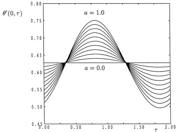
Fig. 2. The rate of heat transfer,  $\theta'(0, \tau)$ , for  $\omega = 1$  with  $a = 0.0, 0.1, \dots, 1.0$ . The solutions represent the periodic flow after the decay of transients.
