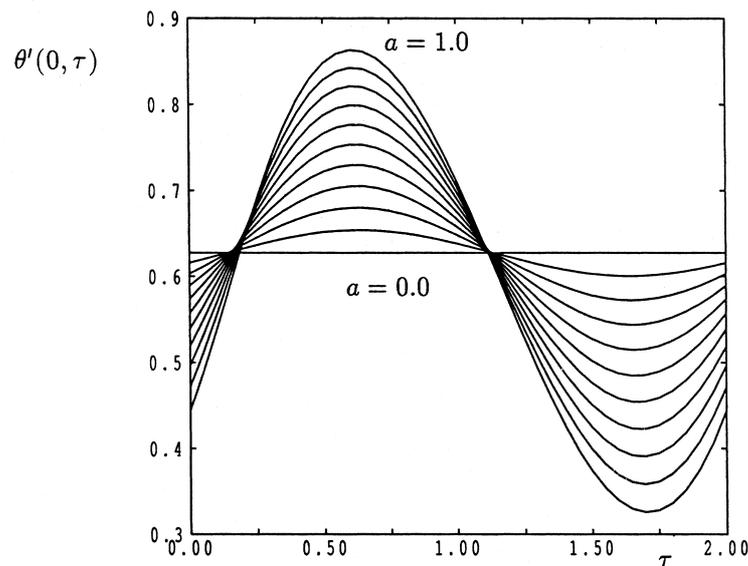
Fig. 3. The rate of heat transfer,  $\theta'(0, \tau)$ , for  $\omega = 0.2$  with  $a = 0.0, 0.1, \dots, 1.0$ . The solutions represent the periodic flow after the decay of transients.
