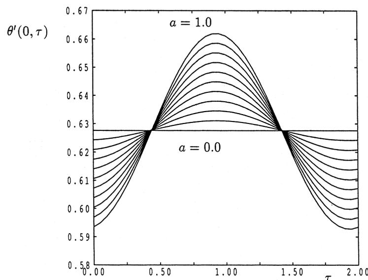
Fig. 1. The rate of heat transfer,  $\theta'(0, \tau)$ , for  $\omega = 5$  with  $a = 0.0, 0.1, \dots, 1.0$ . The solutions represent the periodic flow after the decay of transients.
