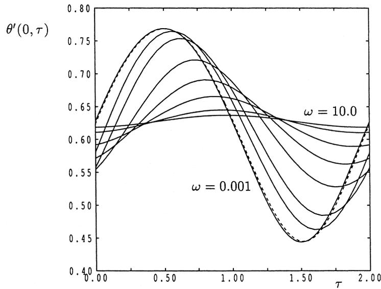
Fig. 4. The rate of heat transfer,  $\theta'(0, \tau)$ , for  $a = 0.5$  with  $\omega = 0.001, 0.01, 0.1, 0.2, 0.5, 1.0, 2.0, 5.0$  and  $10.0$ . The solution for  $\omega = 0.01$  is displayed as a dashed line. The solutions represent the periodic flow after the decay of transients.
