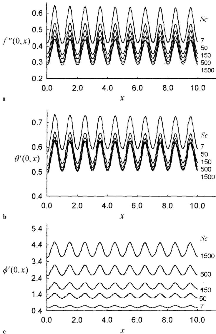
**Fig. 4.** a Skin friction coefficient, b Heat transfer coefficient, c Mass transfer coefficients for different  $Sc$  while  $w = 0.5$  and  $\alpha = 0.2$
