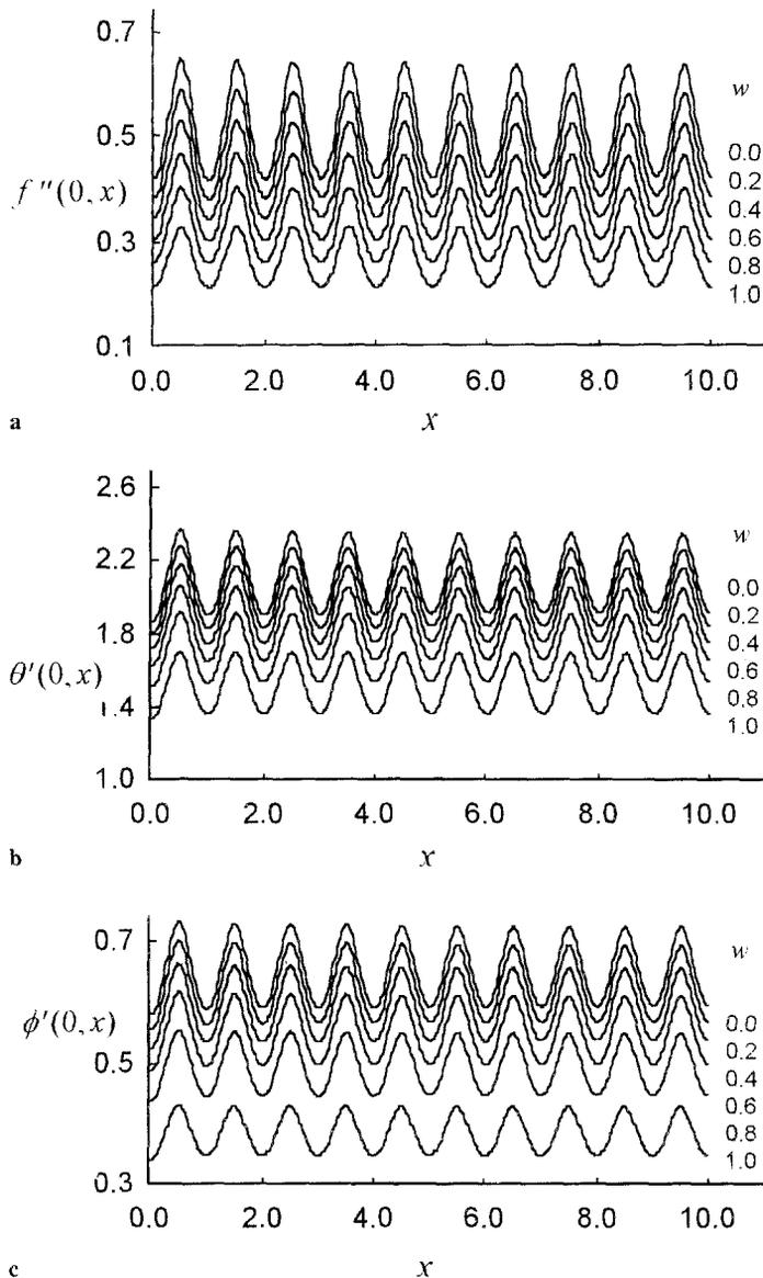
**Fig. 3.** a Skin friction coefficient, b Heat transfer coefficient, c Mass transfer coefficients for different  $w$  while  $Sc = 150$  and  $\alpha = 0.2$
