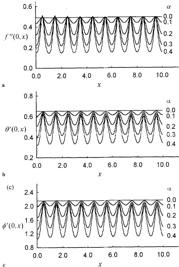
Fig. 2. a Skin friction coefficient, b Heat transfer coefficient, c Mass transfer coefficients for different  $\alpha$  while  $Sc = 150$  and  $w = 0.5$
