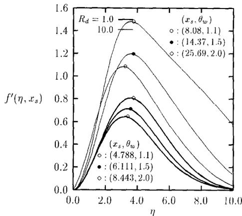
**Fig. 8.** Velocity profiles at the point of separation  $x_s$  for  $R_d = 1.0$  and  $10.0$  and  $\theta_w = 1.1, 1.5$ , and  $2.0$  with  $Pr = 1$  and  $\Lambda = -1.0$
