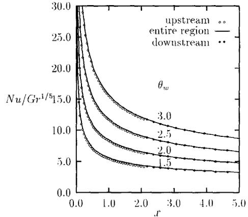
**Fig. 5.** Values of Nusselt number coefficient against  $x$  for different values of  $\theta_w$ , with  $Pr = 1$ ,  $R_d = 10.0$  and  $A = 1.0$
