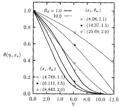
**Fig. 9.** Temperature distribution at the point of separation  $x_s$  for  $R_d = 1.0$  and  $10.0$  and  $\theta_w = 1.1, 1.5$ , and  $2.0$  with  $Pr = 1$  and  $\Lambda = -1.0$
