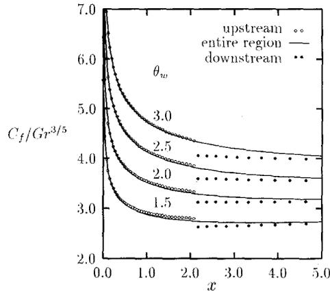
**Fig. 4.** Values of skin-friction coefficient against  $x$  for different values of  $\theta_w$  with  $Pr = 1$ ,  $A = 1.0$  and  $R_d = 10.0$
