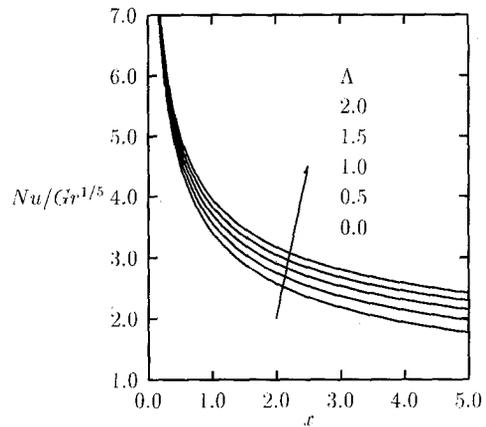
**Fig. 7.** Values of Nusselt number coefficient for different values of  $\Lambda > 0$  with  $Pr = 1$ ,  $R_d = 10.0$  and  $\theta_w = 1.1$
