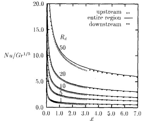
**Fig. 3.** Values of Nusselt number coefficient against  $x$  for different values of  $R_d$  with  $Pr = 1$ ,  $A = 1.0$  and  $\theta_w = 1.1$
