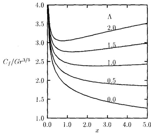
**Fig. 6.** Values of skin-friction coefficient for different values of  $\Lambda > 0$  with  $Pr = 1$ ,  $R_d = 10.0$  and  $\theta_w = 1.1$
