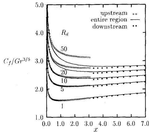
**Fig. 2.** Values of skin-friction coefficient against  $x$  for different values of  $R_d$  with  $Pr = 1$ ,  $A = 1.0$  and  $\theta_w = 1.1$
