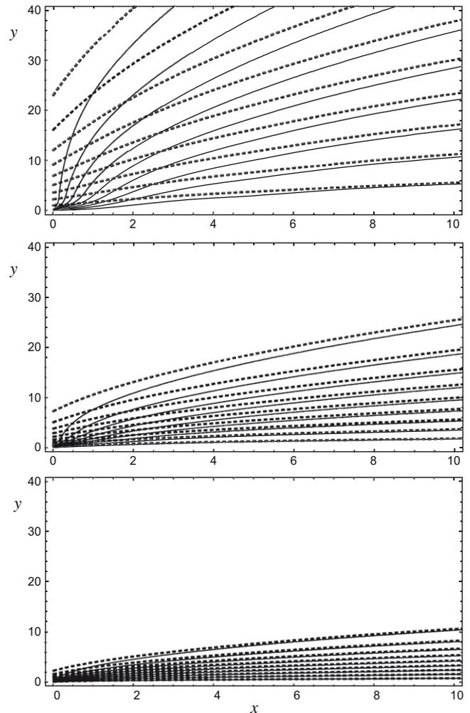
**Fig. 3.** Isotherms for both the solid and fluid phases for  $\gamma = 0.01$  (upper),  $\gamma = 0.1$  (middle),  $\gamma = 1$  (lower). Dashed lines refer to the solid phase and solid lines refer to fluid phase. This figure has a different vertical resolution to that shown in Fig. 2.
