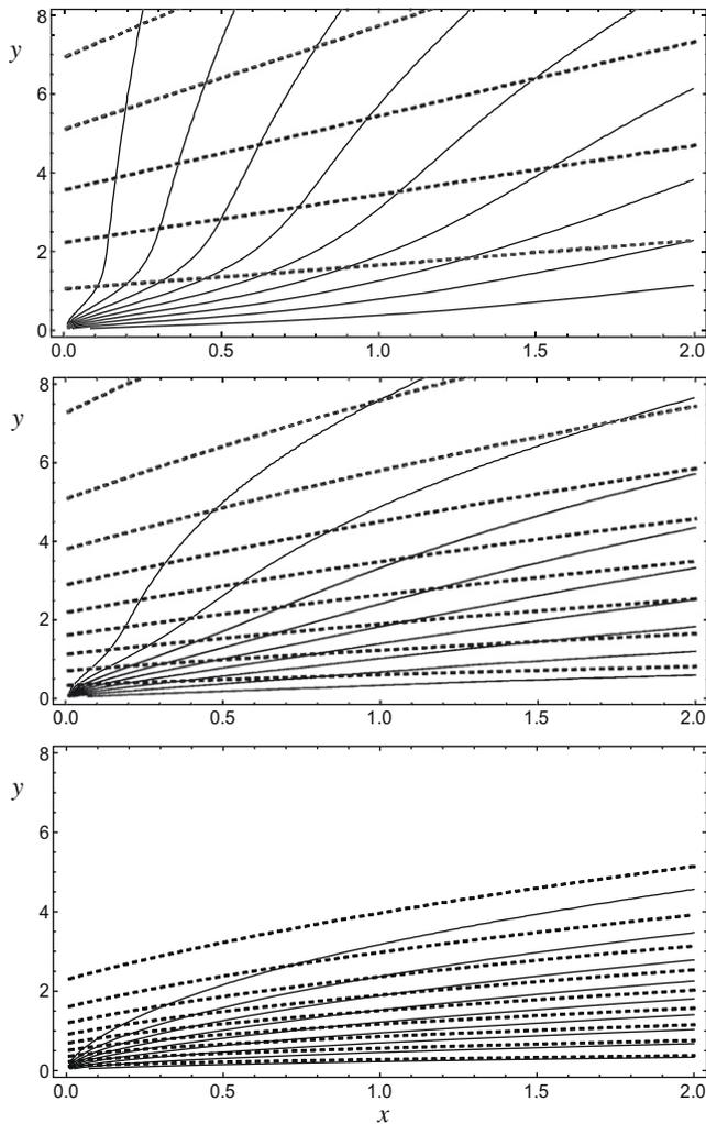
Fig. 4. Isotherms for both the solid and fluid phases for  $\gamma = 0.01$  (upper),  $\gamma = 0.1$  (middle),  $\gamma = 1$  (lower). Dashed lines refer to the solid phase and solid lines refer to fluid phase. This figure has a different vertical resolution to that shown in Fig. 2.
