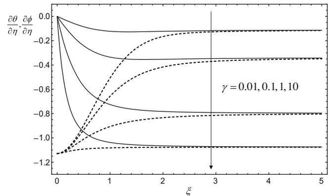
Fig. 5. Variation of the rates of heat transfer,  $\partial \theta / \partial \eta$  and  $\partial \phi / \partial \eta$ , on the plate  $\eta = 0$  versus  $\xi$ , for different values of  $\gamma$ . Dashed lines refer to the solid phase and solid lines to the fluid phase.
