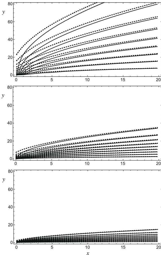
**Fig. 2.** Isotherms for both the solid and fluid phases for  $\gamma = 0.01$  (upper),  $\gamma = 0.1$  (middle),  $\gamma = 1$  (lower). Dashed lines refer to the solid phase and solid lines refer to fluid phase.
