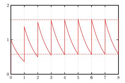
The sudden vertical jumps (all of length, 1) are caused by the successive unit impulses. This graph also shows how quickly the transients decay to form what is the periodic solution for the case when the Shah function is the forcing term.
