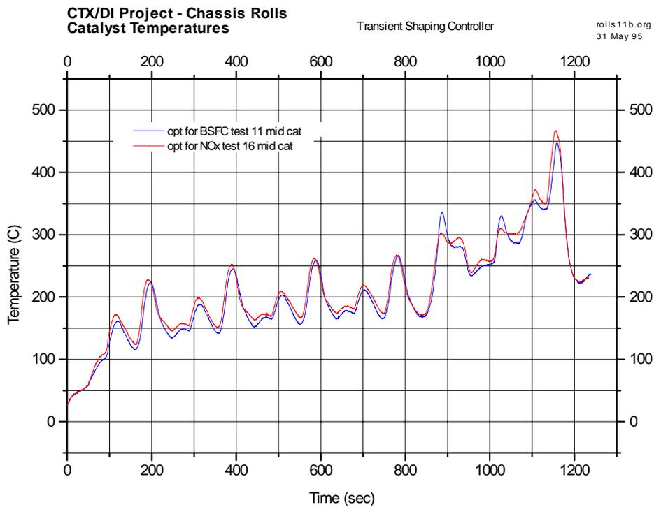
Figure 4.4a - Catalyst temperatures during ECE15 + EUDC
