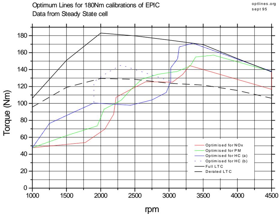
Figure 4.3 - IOLs for 180Nm rating of 1.8DI TCi
