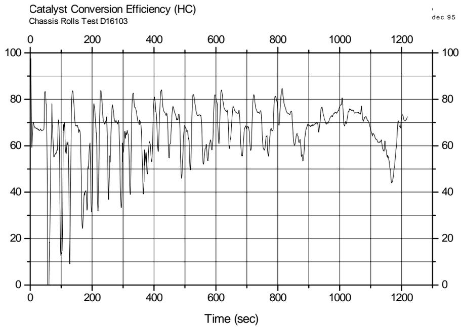
Figure 4.4b - Catalyst conversion efficiency for HC during ECE15 + EUDC
