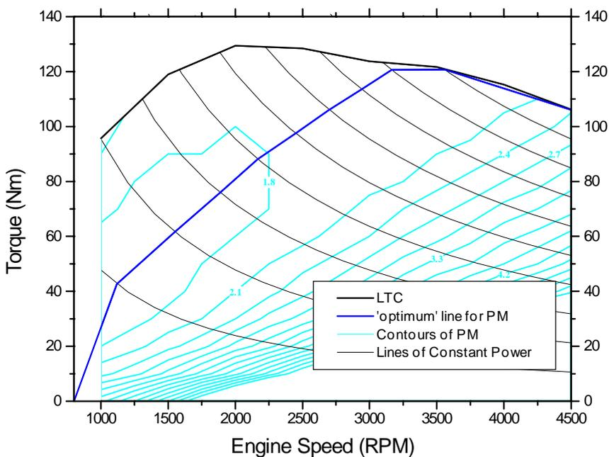
**Figure 4.21 - Optimum line for PM**
