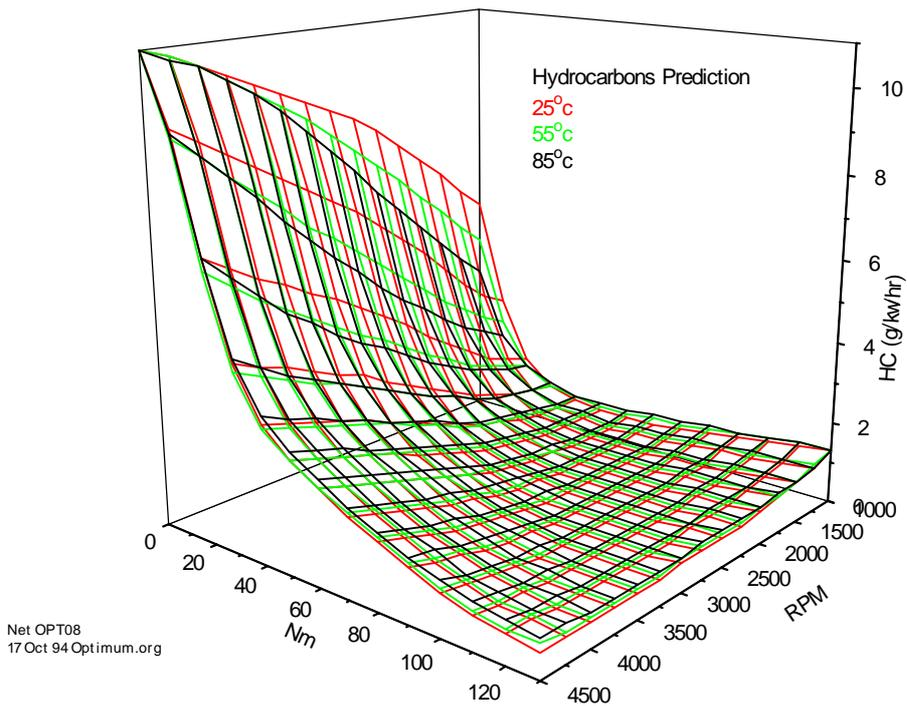
Figure 4.14 - HC predictions at various temperatures
