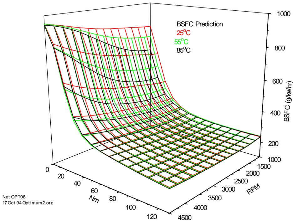
Figure 4.12 - BSFC predictions at various temperatures
