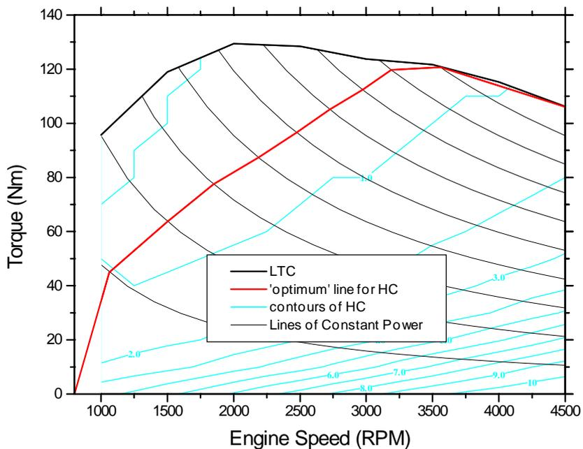
**Figure 4.19 - Optimum line for HC**
