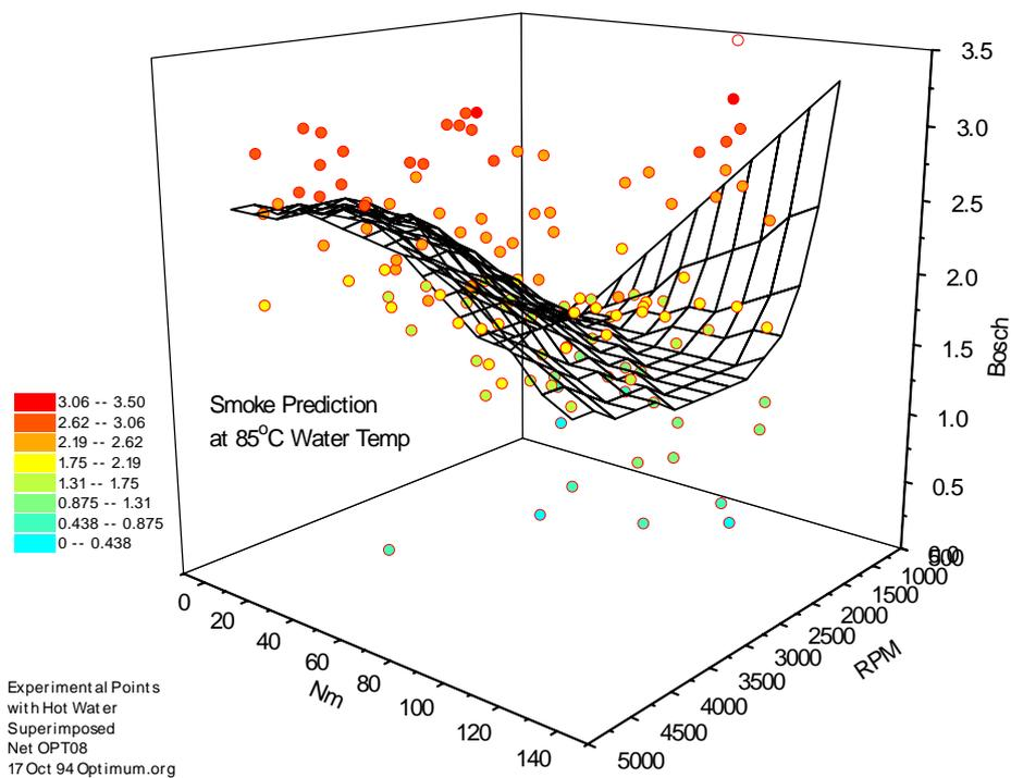
Figure 4.15 - Smoke predictions 85°C water temp
