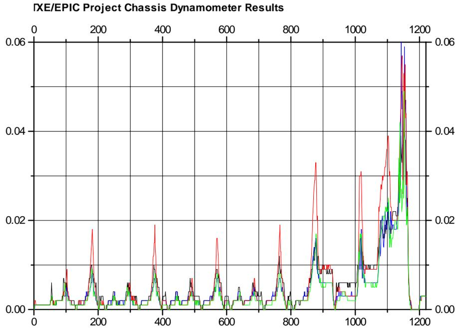
**Figure 4.27 - NOx production during ECE15 + EUDC**
