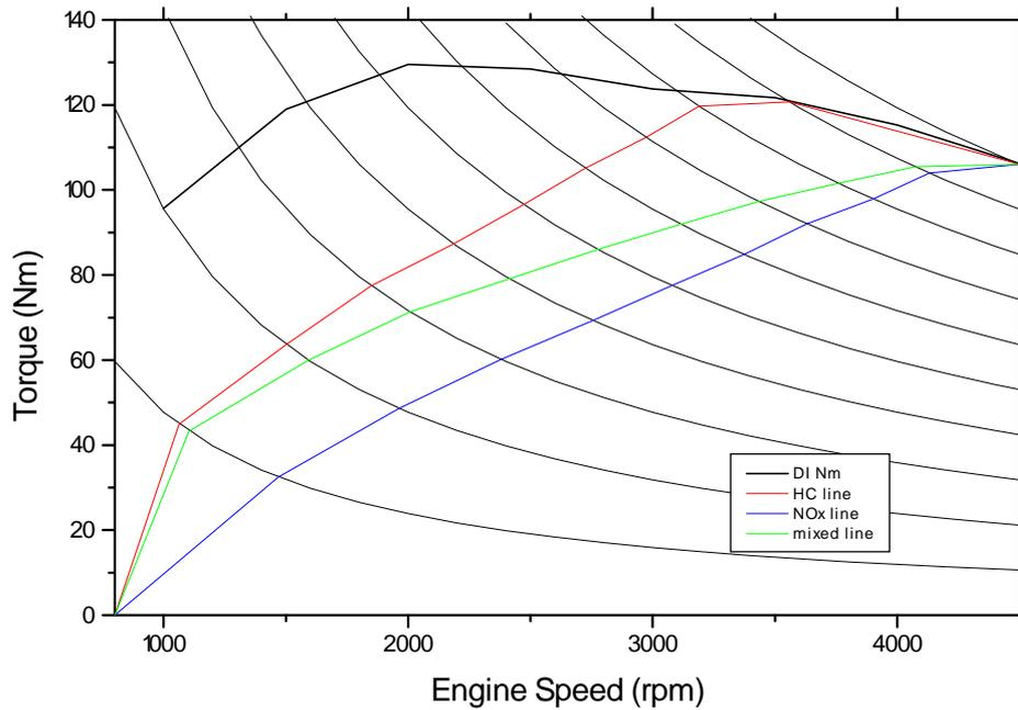
Figure 4.24 - Optimum line for HC & NOx
