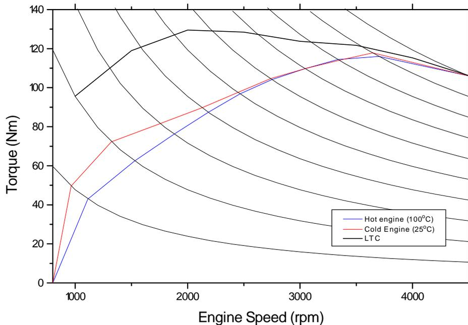
Figure 4.23 - Optimum line with unity weightings for HC, NOx, BSFC & HC
