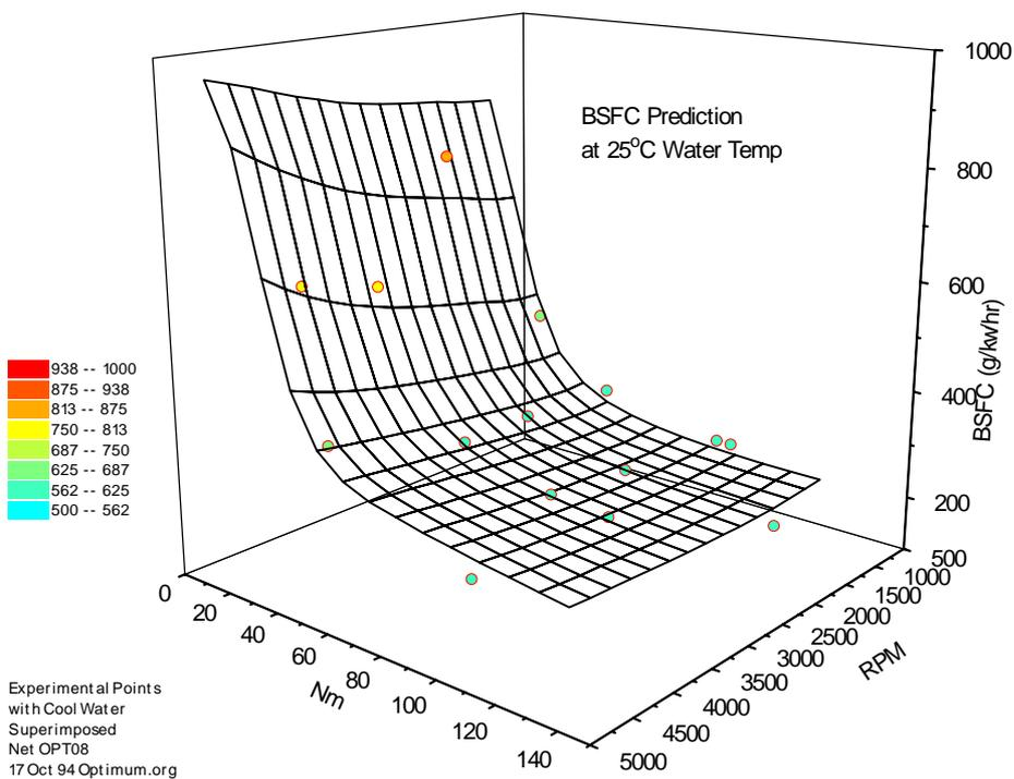
Figure 4.11 - BSFC predictions at 25°C water temp
