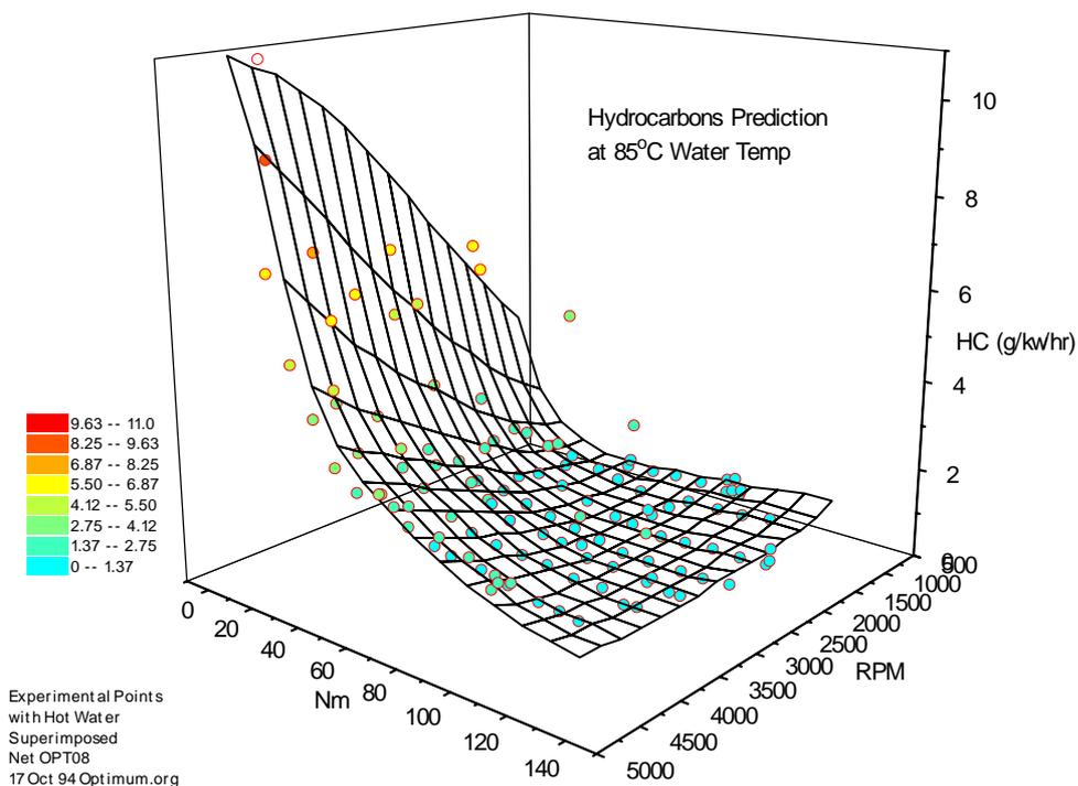
Figure 4.13 - HC predictions 85°C water temp
