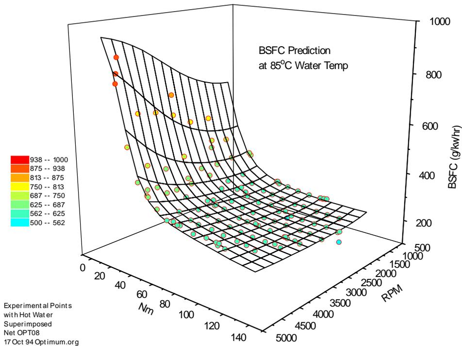
Figure 4.10 - BSFC predictions 85°C water temp
