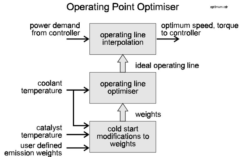
Figure 4.5 - Operating point generator - schematic
