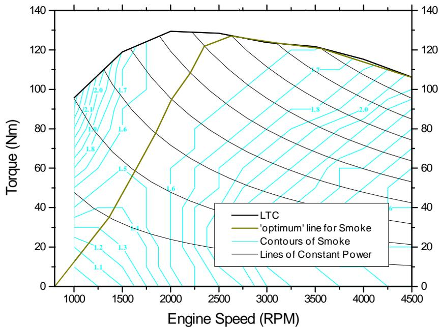
Figure 4.22 - Optimum line for Smoke
