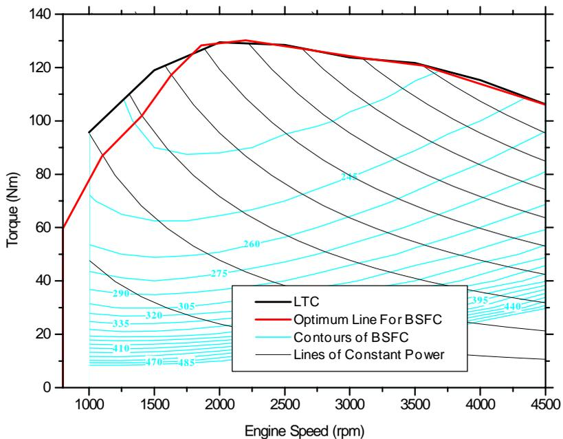
**Figure 4.18 - Optimum line for BSFC**
