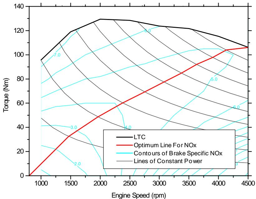
**Figure 4.20 - Optimum line for NOx**
