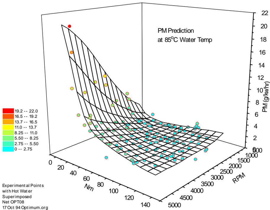
Figure 4.16 - PM predictions 85°C water temp
