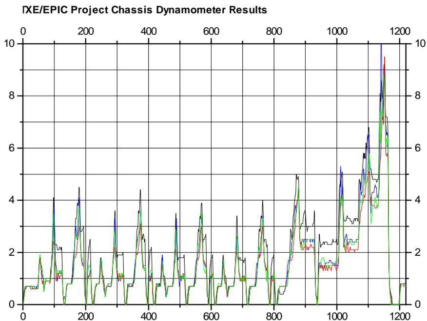
Figure 4.30 - CO<sub>2</sub> production during ECE15 + EUDC
