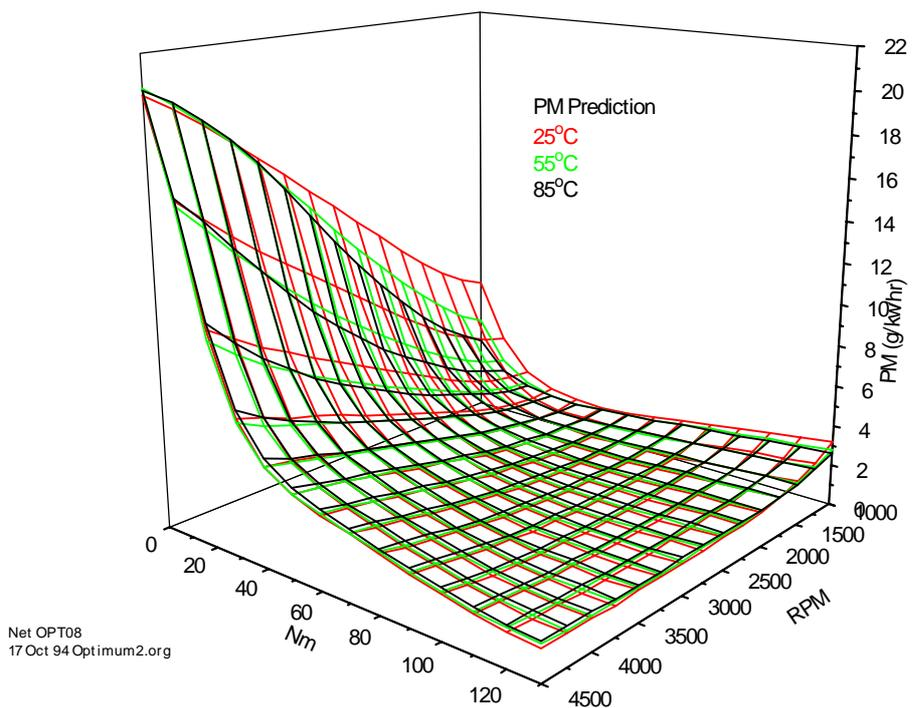
Figure 4.17 - PM predictions at various temperatures
