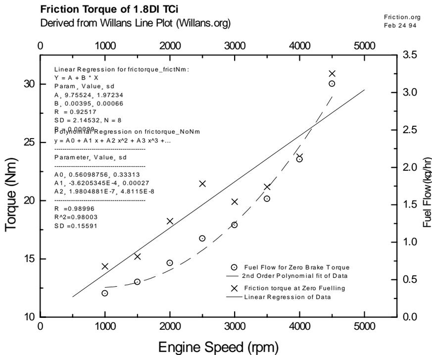
Figure 4.2 - Friction for 1.8DI TCi
