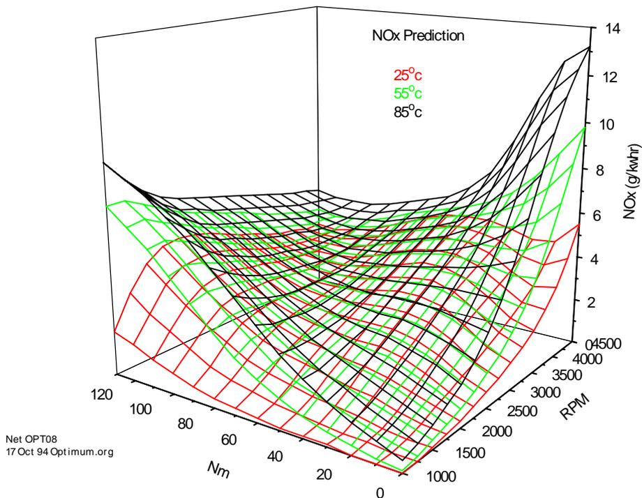
Figure 4.9 - NOx predictions at various temperatures
