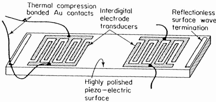
**Figure 11.16** Schematic of a simple surface acoustic wave (SAW) delay line. (From Bristol,<sup>22</sup> Courtesy Proc. IEEE.)
