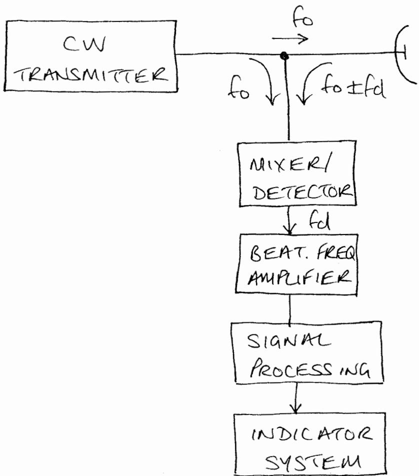
NOTE: THIS IS A HOMODYNE OR "ZERO IF" SYSTEM, AFTER MIXING, WE LOSE THE SIGN OF THE VELOCITY.
