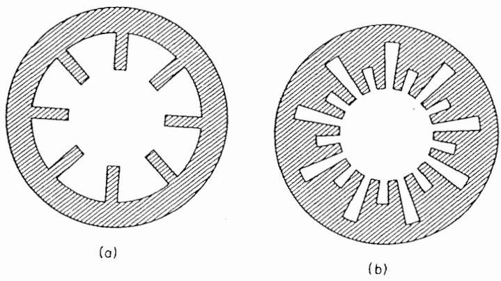
Figure 6.2 Magnetron resonators. (a) Vane type; (b) rising sun, with alternate slot lengths.
