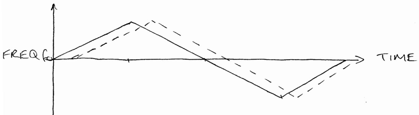
WE CAN DETERMINE THE RANGE BY USING FFT TECHNIQUES TO FIND THE BEAT FREQUENCY AND HENCE DETERMINE THE RANGE
