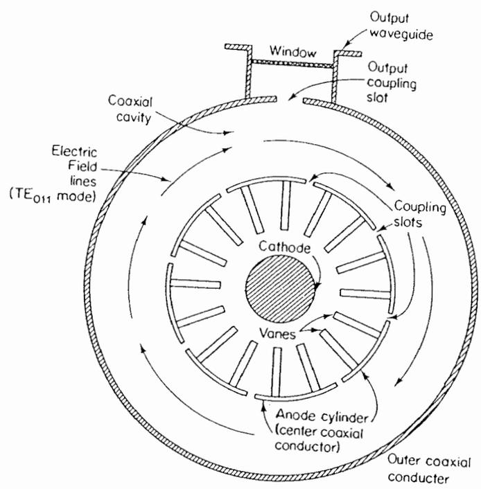
Figure 6.3 Cross-sectional sketch of the coaxial cavity magnetron.
