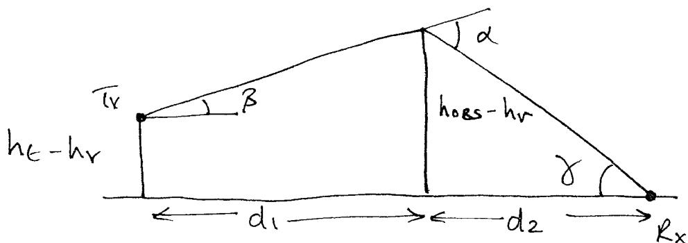
FROM THE EQUATIONS WE DEVELOPED WHEN WE LOOKED AT FRESNEL ZONES, WE KNOW THAT THE EXCESS PATH LOSS IS;
