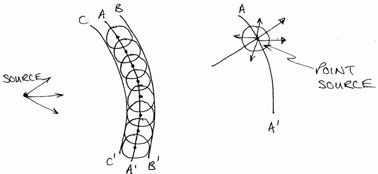
HUYGENS SUGGESTED THAT EACH POINT ON A WAVEFRONT (AA') COULD BE CONSIDERED AS A POINT SOURCE THAT PRODUCES A SECONDARY WAVELET. THESE SOURCES COMBINE TO PRODUCE A NEW WAVEFRONT IN THE DIRECTION OF PROPAGATION (BB') , BUT NOT (CC')
