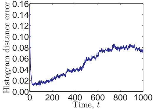
FIG. S.3. *Histogram distance errors for a diffusion simulation using the growth method of Baker et al. [5]. All the particles are initialized in the first interval. Parameters are as follows:  $k_0 = 50$ ,  $\Delta x = 1/k_0$ ,  $D = \Delta x^2$ ,  $r = 0.0001$ .*
